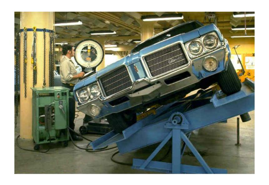
Roll inertia was measured by use of an inverted pendulum. Rick Hill was creator of the inertia test devices. Dave Bubolz is standing by the machine.
