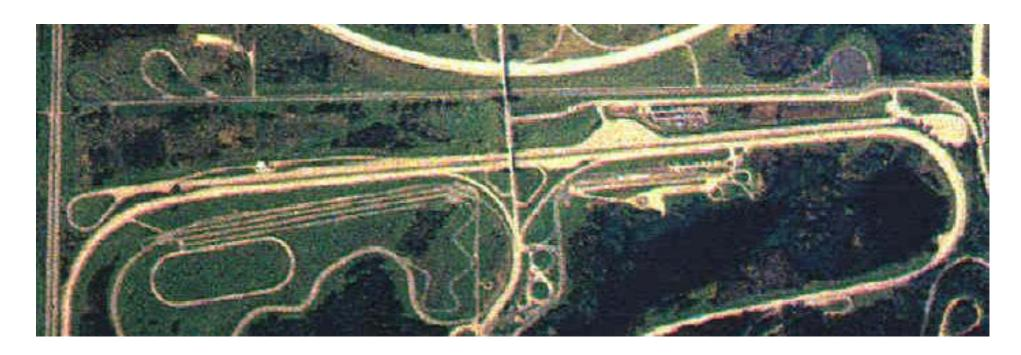
Later on, the Vehicle Dynamics Test Area was built, 67 acres of 6 inch asphalt. This also got a special name, Black Lake, because when it was wet the migrating geese thought it was water and landed pretty hard.
