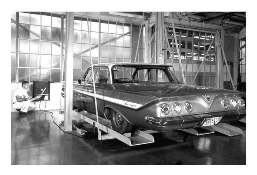
Roll steer and roll rate distribution were measured by a device that transferred water from tanks mounted on a transverse beam fixed on the vehicle. This caused the vehicle to roll, and as it rolled, wheel weight and wheel steer information were recorded.
