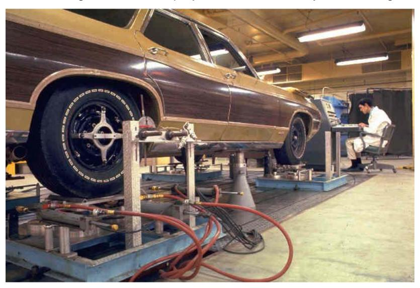
Then a new sophisticated unified test machine was built at Chevrolet, and parameter testing advanced further still. Lloyd Nedley was a key person in this work.
