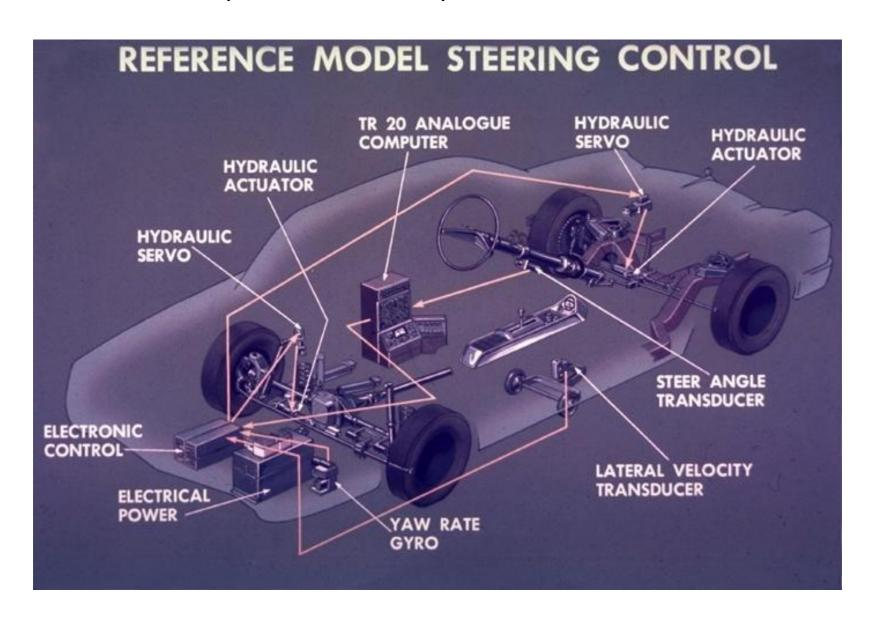
But the size of the VRV car itself and limits on tires and control system bandwidth were constraining. We could not produce Formula 1 handling properties, but there was still a lot of range in handling qualities available for study.
